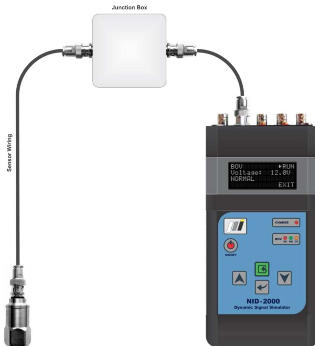
Figure 128 Testing IEPE Sensor including Cables and Junction Box
