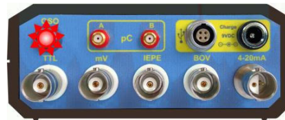
Figure 53 Simulator in the RUN Mode with OSO ® Output Enabled
