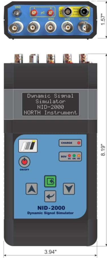
Figure 118 Device dimensions in inches
