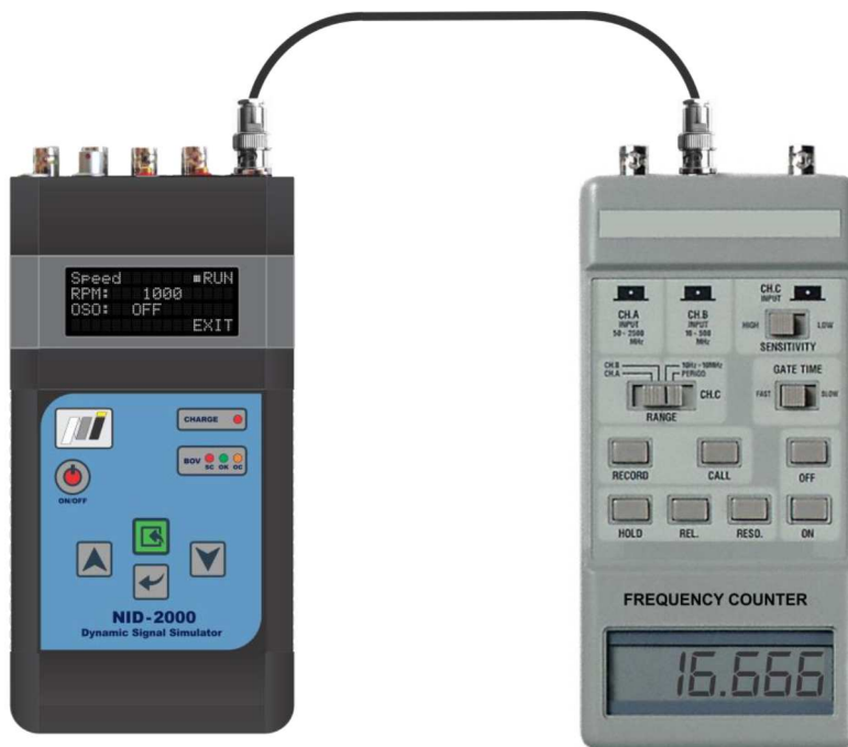
Figure 126 Testing Frequency Counter
