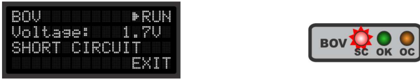
Figure 59 BOV Test - SHORT CIRCUIT
