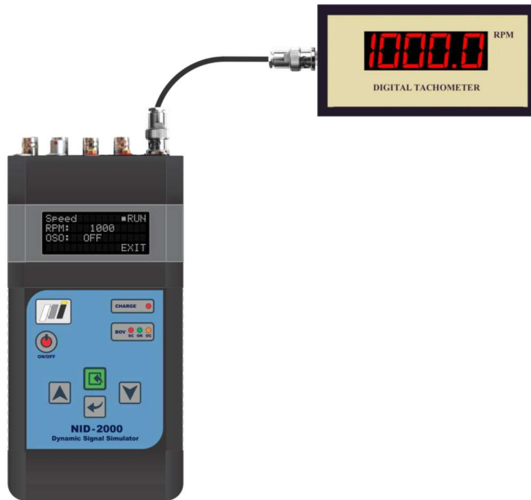
Figure 124 Testing RPM Meter
