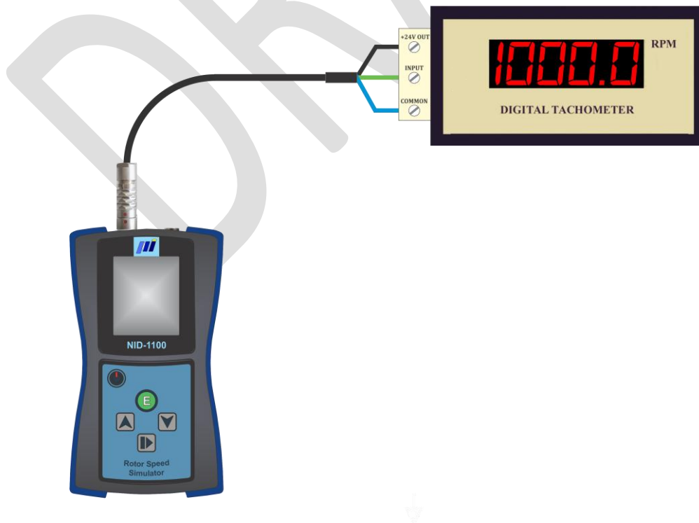
Figure 67 - Using RPM Voltage Output (Positive DC Power Supply)
